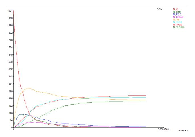
In this simulation 1024 nodes self-assemble; the bottom 4 traces are the 4 different 'root' states, and the 4 top traces are the 4 different 'non-root' states. The root states go to zero because of cycles being formed; the population appears to converge to a roughly equal mixture of the 4 non-root states. (Why?)
