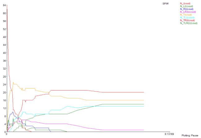
Here we simulate 64 nodes assembling into a single tree: in the end, there is a single copy of a root node N\_LR.
