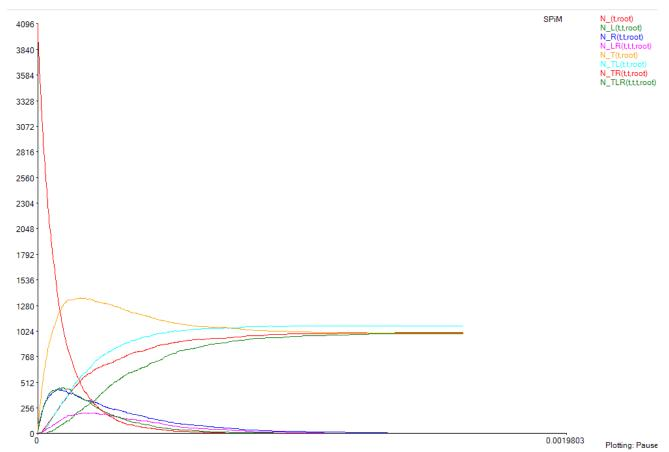
Same, with 4096 nodes (there is a single copy of a root node left at the bottom, which happens to be N\_R). When you change the number of nodes, you should readjust the sampling parameters in "directive sample x y" so that x is close to the interval you mean to plot, and y is e.g. 10000 (number of sample points), or you may not have enough sample points in your interval.
